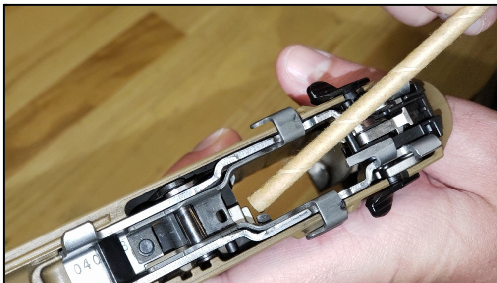
Takedown safety lever in the forward position to clear the magazine well
